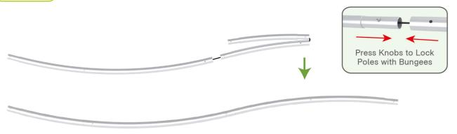
STEP 02 Connect long poles with corner poles according to labelings.
