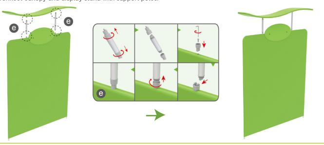
STEP 03 Insert display stands onto feet by pressing their knobs.
