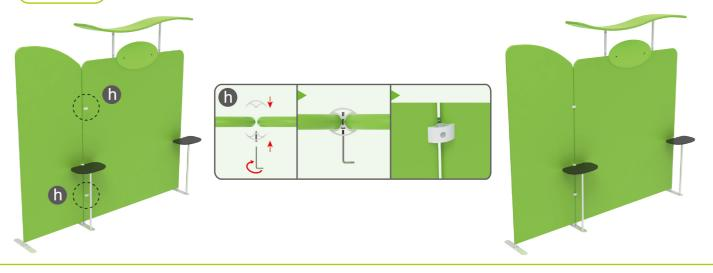
STEP 06 Screw light clips at top of display stands, slide lights onto them and adjust their direction.
