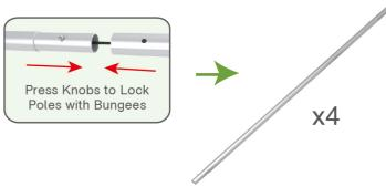
STEP 02 Connect long poles with corner poles according to labelings.
